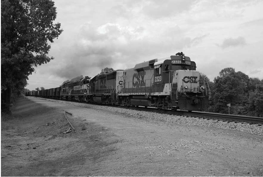
Two Red Geeps of Wisconsin Southern trail mother and slug CSX units on a south-bound ballast train near Hopkinsville. Photo by Chuck Hinrichs
